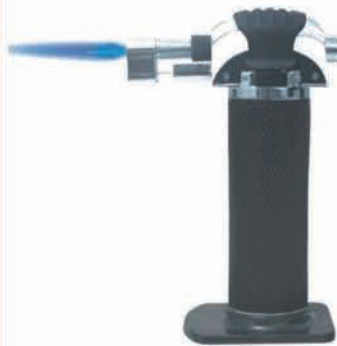
#K2002 Micro Torch, 851# 焊枪 Max. Temperature: 1300°/2450°F uses butane fuel, Capacity: 90ml
