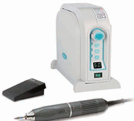
S01 Marathon Multi 600, Brushless Speed range: 1,000-50,000 rpm, Torque: 7.8Ncm Easy Changeable to Knee, control or Desktop, Made in Korea S01 韩国世洋600无碳刷打磨机, 5万转
